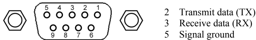
Fig. 5.3: RS-232 port pinout.
