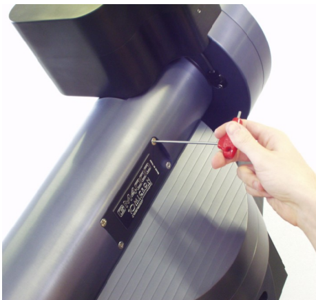
Fig. 4.10: Accessing the declination axis hole.
