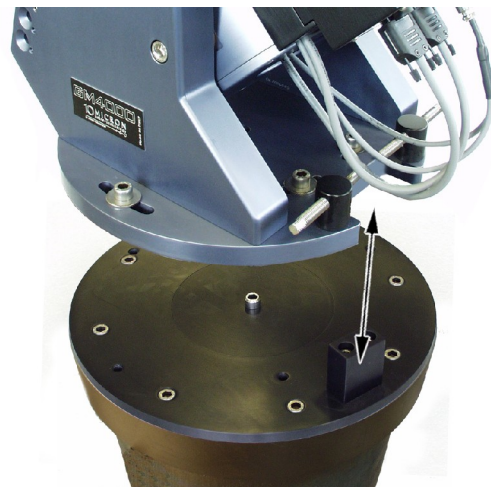
Fig. 4.8: Mount and base adapter alignment.
