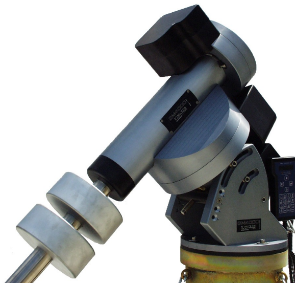
Fig. 4.14: This is the right position to attach the counterweights and the telescope.
