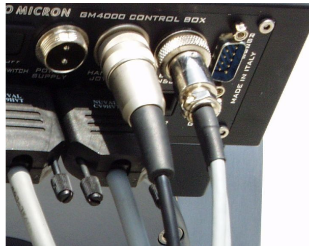
Fig. 5.13: Hand pad cable connection.
